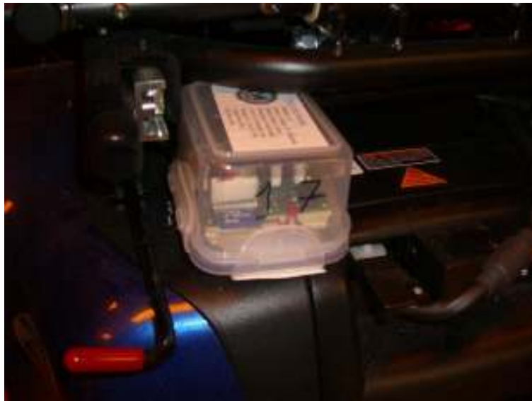
Figure 12: Data Logger Attached to a Wheelchair
