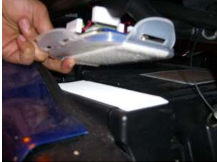
Figure 11: Velcro Adhered to the Wheelchair and the Data Logger for Coupling
